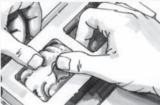
Curing Castaldo Silicone Jewelry Molding Rubber involves no mixing, limited working times or de-bubblizing. Simply put it in your vulcanizer at 200°F (93°C) for 15 minutes.
