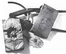
Normally a mold release agent is not needed, although some workers prefer to use talcum powder or a silicone or Teflon® spray. If talcum powder is used, avoid a buildup of powder in the mold cavity, cleaning it if necessary with an air gun or a soap and water solution.
