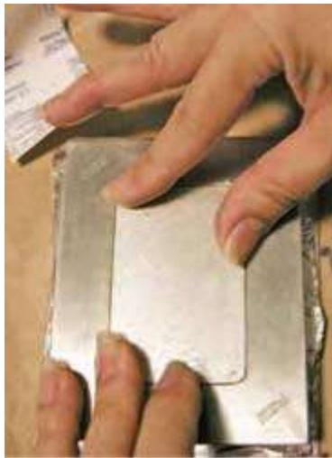
If there is a definite drop off between the rubber and the frame surface, add a thick plate or possibly more than one plate. You want the plate surface to be just slightly above the frame surface. If you put too little pressure, you'll get a spongy mold with incomplete fill/fit. If you put too much pressure, you'll cause too much displacement, causing rubber to ooze out, and the keys and the model to shift. Identifying correct pressure comes with experience.
