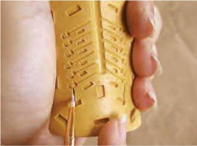
Flex the mold to open up the slits. Take a fine brush and dust a little powder into the slits, not on the rest of the mold. Use compressed air to remove the extra powder. These slits, with a little powder, will let displaced air escape and allow wax to flow more easily into the mold cavity.
