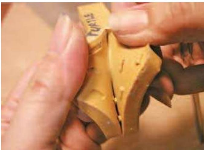
chain to hold one end of the mold, cut the mold apart with a scalpel. Pull the rubber as you're cutting, so it releases away from the model. Don't pull too hard or the rubber might tear.
