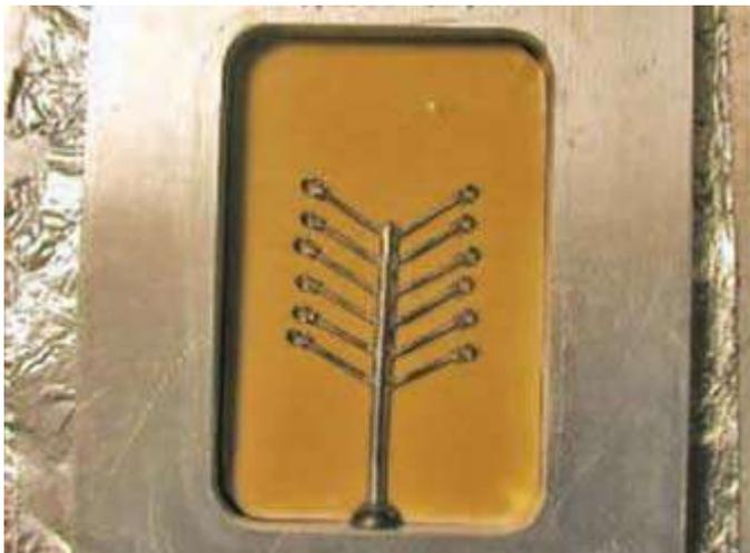
and along the sides about 1/8" from the edge and base former. If the keys are too close to the side, they may shift during vulcanization and
