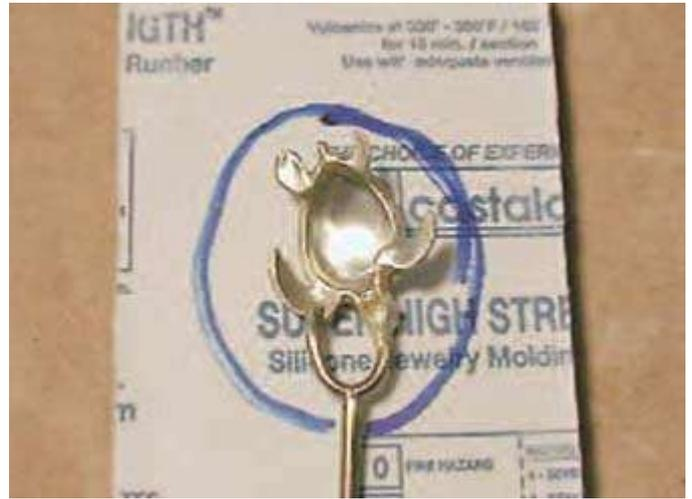
Remove the model, take an X-Acto knife and cut through the safety paper on the line just drawn. Remove the safety paper outside of the model area and place the rubber slice into a prepared frame assembly. Press in a sprue base former, and place keys in the perimeter and base area.
