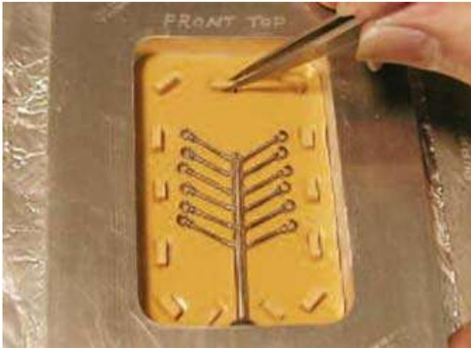
break through the outer edges of the mold. The keys, standing on their bondable, powder-free cut edges, are pressed halfway into the rubber. Try to use keys that will cause even and symmetrical displacement. Don't use skinny keys on one side and fat ones on the opposite side, because the displacement will be uneven, and the model might shift out of place.
