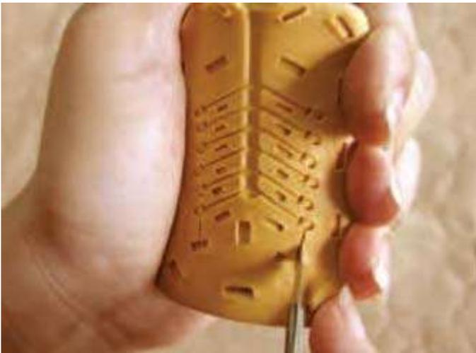
NOTE: How many, how deep, and the direction of the cuts affect how the mold flexes open. An excessive slit could cause the mold half to crack open too much when flexed, and break the wax model. The general rule of thumb is to cut the minimum to achieve wax fill. This minimizes flashing, flexing problems, and preserves the durability and strength of the mold. Don't despair if you make venting
