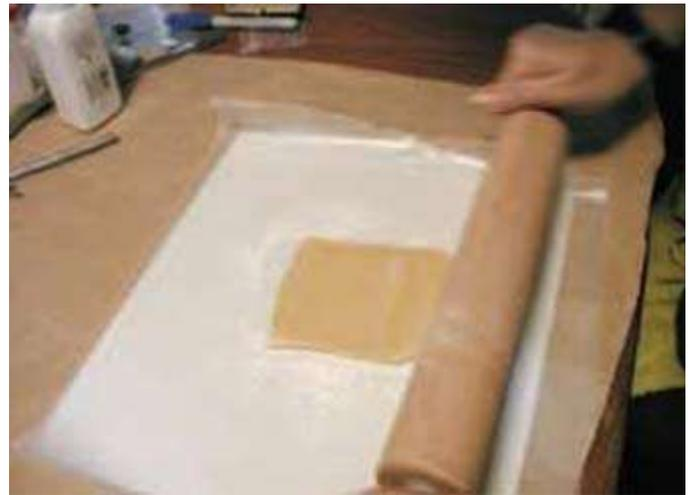
After you've rolled out an even thickness, place pressure plates on the sheet to serve as templates, and cut around them with a dull butter knife. Powder the cut edges of the rubber
