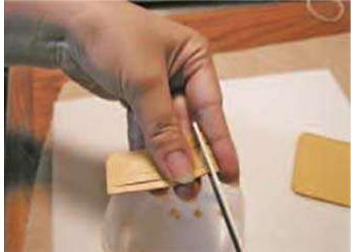
cut across the strips, and by the thickness of the sheets. When you've cut to the anchor edge, discard it. When I make keys, I generally use one of my frames with a larger opening or a double frame so I can mass produce the keys. I avoid frames thicker than 5/8" to 3/4" because tall stacks are more difficult to remove. Within a stack, I can make sheets of different thicknesses. I separate my keys into containers by size.
