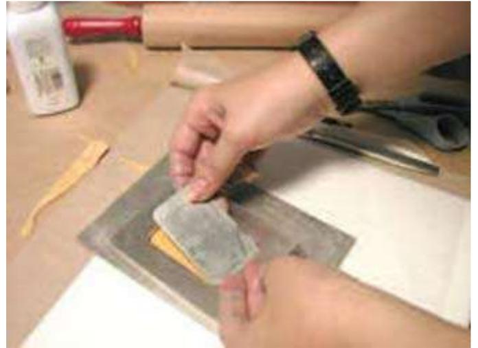
Place sheets of rubber, alternated with pressure plates, into the frame until it is firmly filled up just beyond the top surface. Cover with another piece of foil and the second frame plate. This mold frame sandwich is placed into a 330°F
