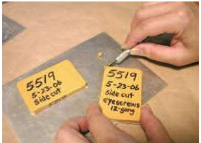
make the marking permanent. If you mark after the rubber is vulcanized, the marks tend to rub off. NOTE: I usually record the mold number, the date, and other pertinent notations. I mark
