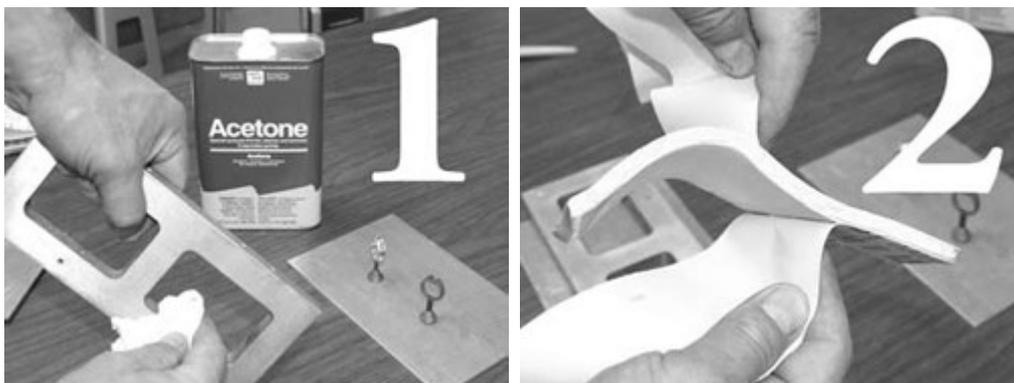
(Photo1). VLT strips are thicker than the natural rubber strips. VLT is about 7mm thick while the natural rubber is 3 – 4mm thick, which means you are only handling three sheets to fill a 19mm mold frame not six or seven. Pull off the protective wax paper covering from both sides of the material (Photo 2). Lay the sheet over the mold frame and with your fingers push the material against the frame to mark the sheet for cutting (Photo 3).
