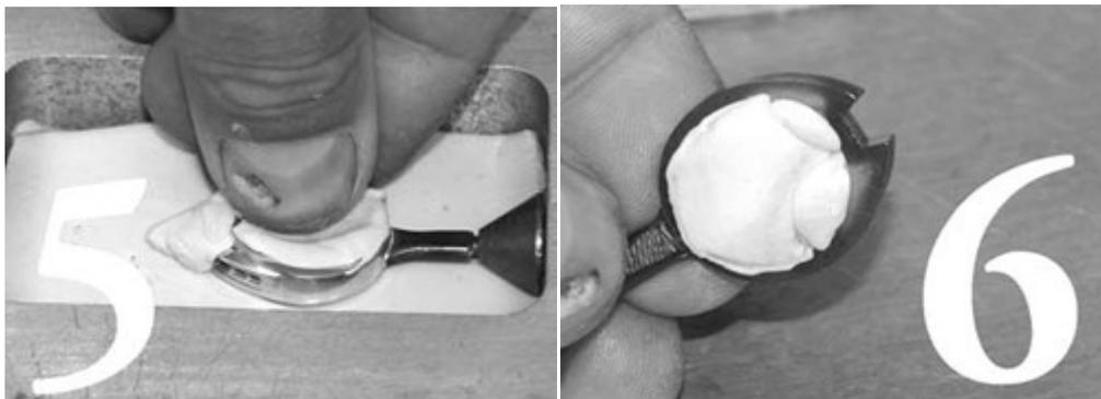
I did no special preparation to the metal model before making the mold. I had no problems with the VLT sticking to the surface of the ring. With VLT you are able to make molds of plastic resin models created by CAD-CAM rapid prototyping systems as well as traditional wax carvings. This saves time and an extra step by not having to cast a model before producing a mold. In this experiment I used a ring model carved from a Matt hard green wax tube.
