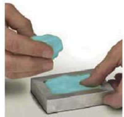
Figure 2: Placing the Objet model inside the mold.
