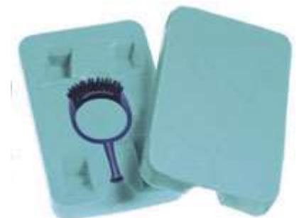
Figure 3: Finished mold can be complex with even spiral plugs.
