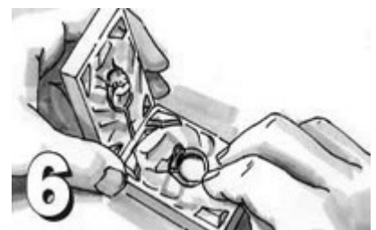
Parting lines are easily controlled and corrected by hand when used with the powder separation.
