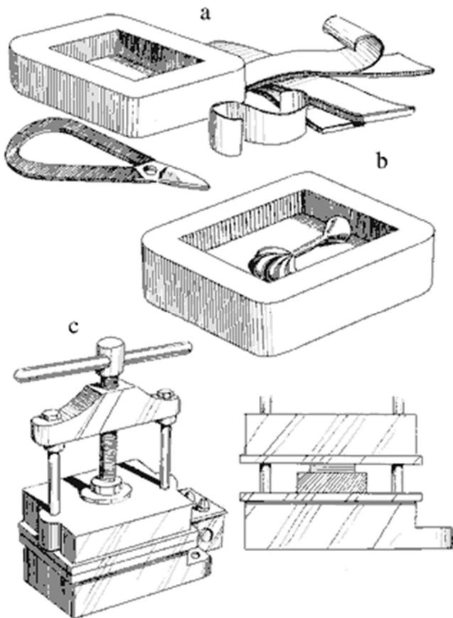
So first the piece must be appraised by the mold-maker, not only for the quality of the rubber it demands, but also for the approach he will eventually take to cut it from the vulcanized mold. After this has been done, the chosen rubber is cut to fit into an aluminum or zinc-magnesium frame, packed down in layers, until somewhat more than half the frame is completely filled with the rubber [Fig. 1.5a].
