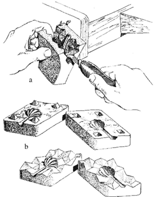
hemisphere, and removal from the mold is an easy matter [Fig. 1.7b]. After polishing, the two halves are soldered together and the bead is done. This same principle applies to any hollow, fully formed three-dimensional object. It must be cast in two halves; the two halves reproduced in the rubber mold and, then, soldered together.
