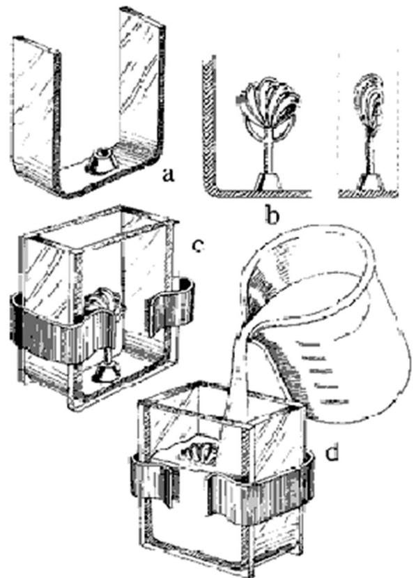
In the trade, this new approach to mold-making is given a variety of names: R.T.V's (room temperature vulcanized molds), cold molds, or silicon molds. However, not all cold molds are silicon-based, some are polyurethane, and not all silicon molds are cold molds. Therefore, for the
