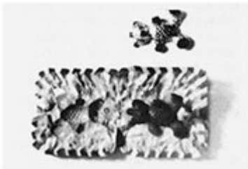
12. Metal master is at top, wax reproduction at right, hollow half-mold in rubber is at left.
