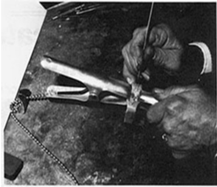
8. Serrated clamps act as fingersavers when rubber is cut with a very sharp X-acto or razor blade.
