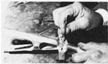
9. Slit in rubber is probed carefully to located metal master, so cut can be centered on the master.
