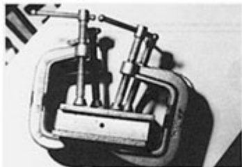
6. C-clamps hold side plates, but special clamps may work better.
