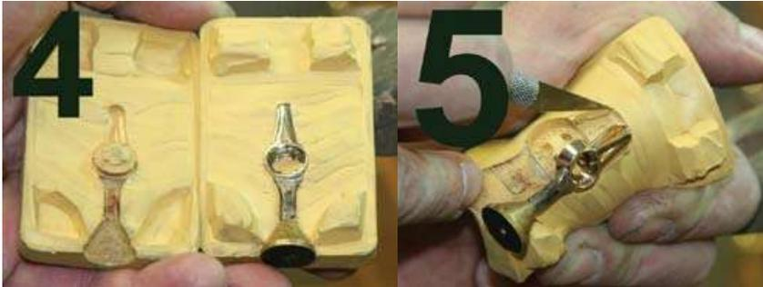
As we come to the body of this pendant, I stretch and pull the rubber as far as possible to cut this inside body plug even with the inside top of the pendant. Photo 3 shows the mold halves still attached at one end with the center plug on one side and the pendant on the other side. At this point I finish cutting the mold keys at the top of the mold before cutting the
