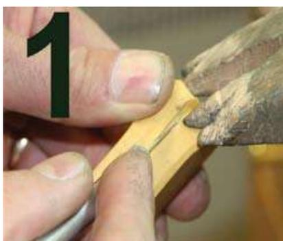
I start by cutting an 1/8” deep cut around the center perimeter of the mold (Photo 1). This is my start point for cutting my “keys or mold locks.” The “keys” must be cut deep enough so the mold will not slide or slip during wax injection. Rounded keys have a tendency to slip during injection. I have found flat topped keys with sharp corners hold the best during injection, minimizing mold lines in the injected pattern.
