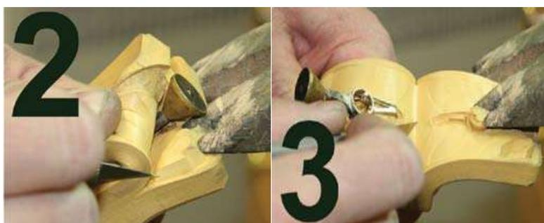
I cut the first two keys near the sprue and usually cut the two keys on the other end of the mold after cutting around the model. To cut a key, I lift the edge of a mold half at the perimeter cut I made earlier. I then angle my blade down at about fifty to sixty degrees and cut a slot just inside the mold perimeter about 3/16” to 1/4” deep around
