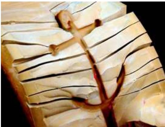
1. This anchor mold, which has no vent cuts, was filled at 10 psi with a conventional wax injector. The flash surrounding the pattern is a result of the trapped air being forced out through the parting cut.
