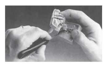
Castaldo White Label®, the less expensive of our two grades, has a high concentration of pure natural gum rubber, which makes it soft and pliable, qualities that the experienced mold-cutter values in his efforts to produce high-quality molds in the shortest reasonable time.
