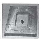
Most of the rubber is available in strips the width of the mold frame cutout, with a plastic sheet on both sides. The rubber must be clean, and free of foreign matter adhering to it, or else these imperfections will turn up in the rubber mold and prevent the layers of rubber from adhering to each other. Therefore the plastic is attached to both sides, and should be left until the moment you use it in the frames.
